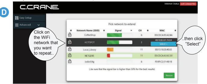
NOTE: For best performance, your signal should be higher than 50%. For a better signal, try adjusting the orientation and placement of the USB antenna - then click "Rescan" to see if the signal is higher.
