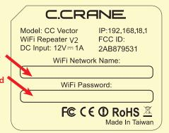
After confirming you have completed Step "B", open the Internet Browser screen on your device and enter **192.168.18.1** into the Address Bar. Press "Enter" on your keyboard.
